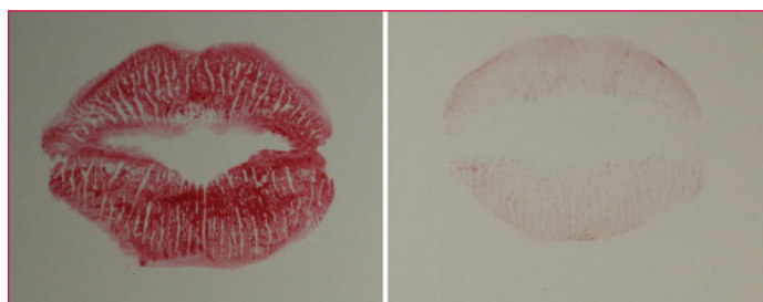
Lip glosses with (a) & without (b) silicone elastomers as plasticisers
