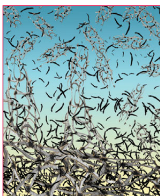
The elastomer dispersion acts as a 'spacer' in the thermoplastic
