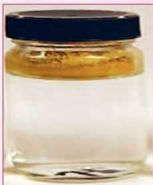
Figure 1 – An image showing the hydrophobic nature of yellow iron oxide treated with NJE.
